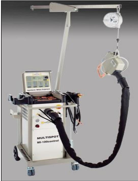
The MULTISPOT® MI-100control is specifically designed for high-strength steels such as Boron, USIBOR, TRIP, TWIP, and XIP.
