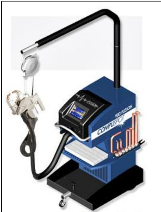
This unit is designed to weld modern ultra-high strength dual phase and boron steels, with up to 630 daN (1,386lbf) of tip pressure and 14,000 amps of welding current.
